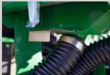
A simple slide gate below each seed box shuts off seed for quick meter change without draining boxes.
