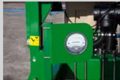
Large pressure gauge located on the front of the planter provides quick confirmation of air flow to meters.
