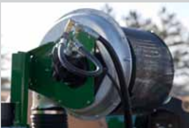
The hydraulic fan provides positive air pressure to meter seeds without worry of vacuum leaks.
