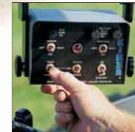
Cab-installed control console, with backlit face, controls folding and row marker functions.
