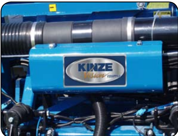
CAN Bus Modules with Cover
