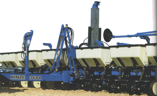
3600 Twin-Line® "T" 12 Row N (30") with Dry Fertilizer Package and HD Single Disc Openers
