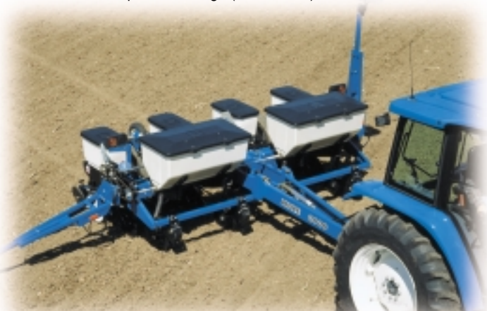
3000 Pull Type 4 Row W (36"-38") with Dry Fertilizer Package and Double Disc Openers
