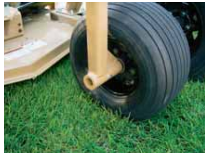
Gauge wheels feature bolt in spindles for ease of replacement, and 18" tires leaving a light weight footprint.
