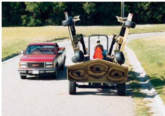
Transport width of 9'6" allows for safe transport from site to site.
