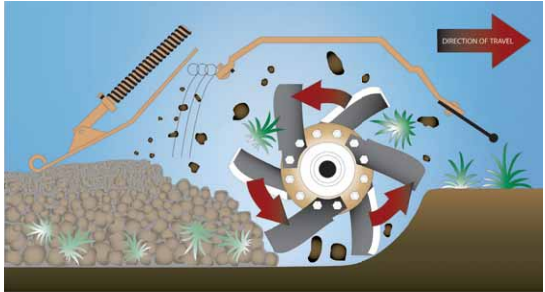
The reverse rotation of the tiller tines forces the tiller in the ground, preventing "walking" on hard ground. Once it's in, it stays put!
