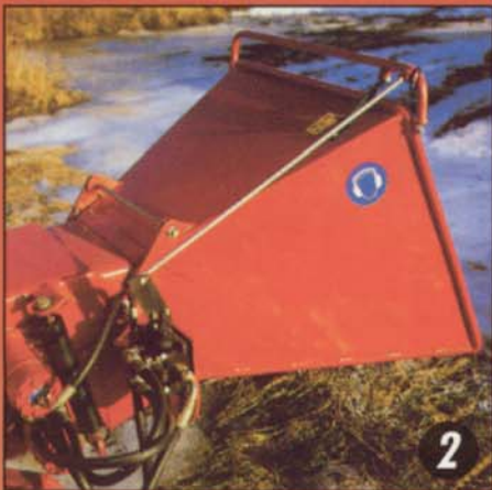
Fig. 1. The DC 100 HFS features a complete integral hydraulic system with pump and oil reservoir for driving the feed rollers.
