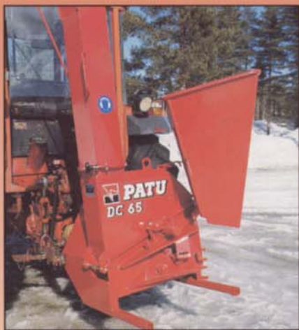
The feed chute can be folded up and latched. This makes road transport easy.
