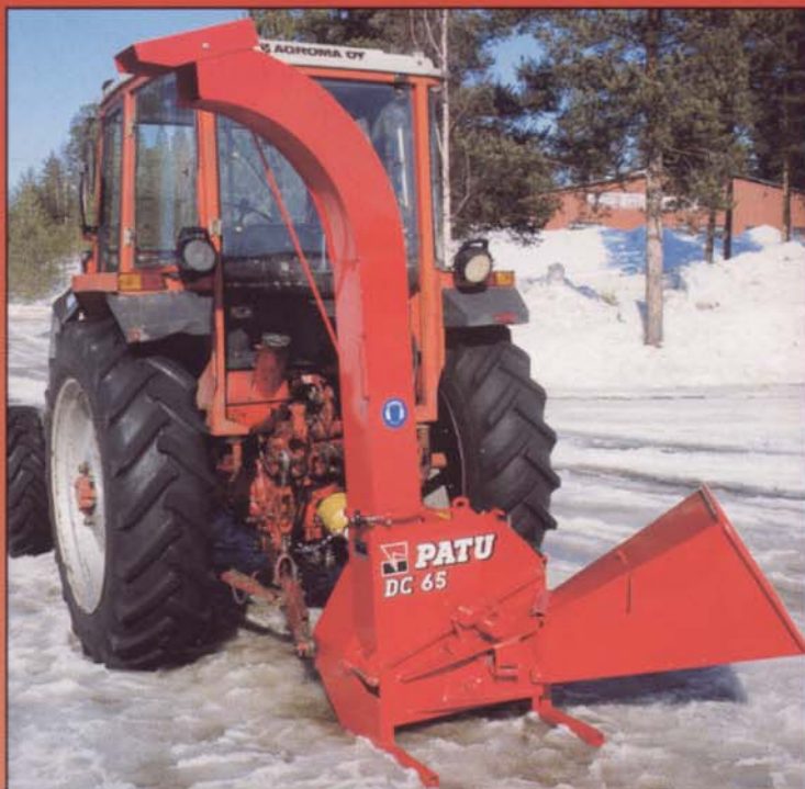
The Patu DC 65 MF has a powerful manual feed. The knives pull in most of the material with no pushing by the operator. A slab even 9" (225 mm) wide can be fed into the DC 65 MF.
