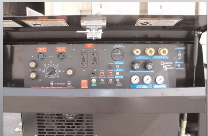
Integrated control panel with hydraulics.
