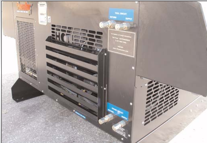
Tool circuit and crane circuit hydraulic connectors.
