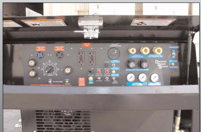
Integrated control panel with hydraulics.
