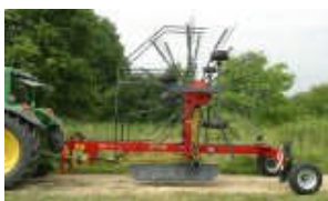
The mainframe can be hydraulically lowered for transport
