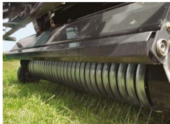
The crop baffle plate and the large guide wheels give a clean raking job
