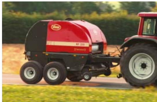
Tandem axle allows forward speeds up to 60 km/h.
