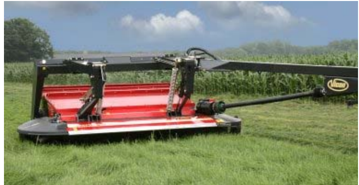
The new EXTRA 832T with new cutterbar and steel tine conditioners
